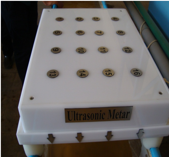
Photo (2) View of measuring devices (Ultrasonic devices - multi spots).
